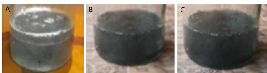
Figure 5: Different length carbon fiber dispersing in PVA solution (a) 3 mm, (b) 6 mm, (c) 10 mm.
