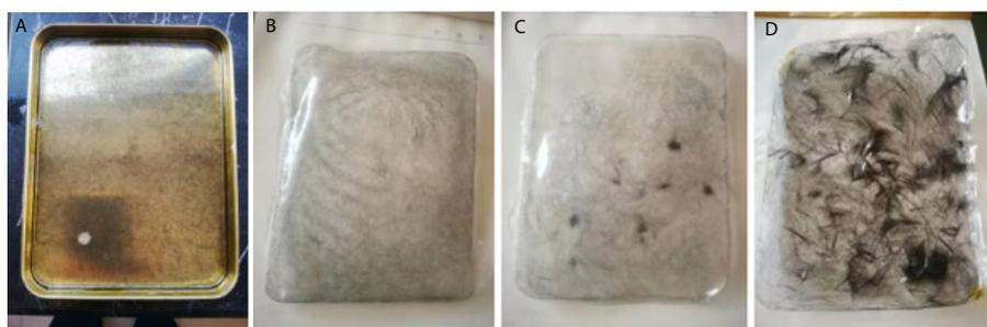
Figure 6: Casted film with carbon fiber in PVA solution: (a) Casting mold. (b) Film with 3mm CF filament. (c) Film with 6mm CF filament. (d) Film with 10mm CF filament.
