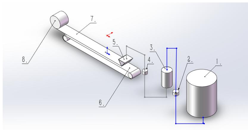
**Figure 12:** Fabrication machine for basic flexible conductive PVA-CF. 1: Mixer drum for mixing and blending of PVA, CF and glycerin. 2 & 4: pump. 3: Vacuum cavitation cylinder. 5: Horizontal slit funnel. 6: Heated conveyor steel belt. 7: PVA-CF film. 8: Winding machine.
