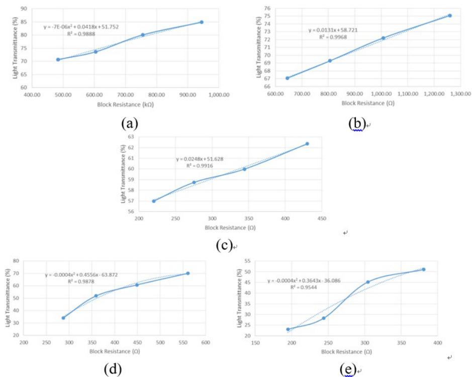
**Figure 9:** the relationship on the sample for Light Transmissivity vs. Block Resistance with Equations for CF-PVA. (a) Sample-01, CF:PVA of 0.1:30, (b) Sample-02, CF:PVA of 0.2:30, (c) Sample-03, CF:PVA of 0.3:30, (d) Sample-04, CF:PVA of 0.6:30, (e) Sample-05, CF:PVA of 1.0:30.
