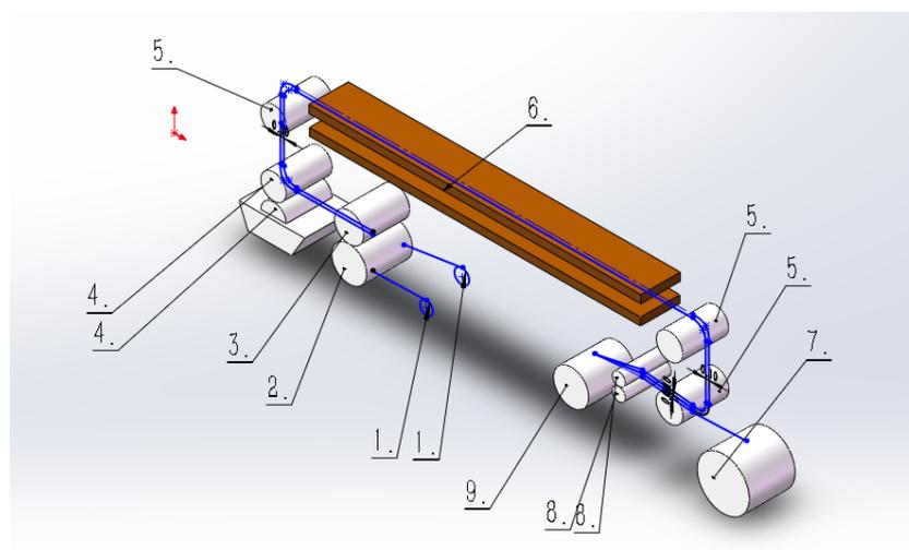
**Figure 13:** Modified food packaging machine for application of metal copper foil strips and protection laminate. Blue line indicates the feed path of the film. 1: current-carrying, 2: PVA-CF film roller, 3: Top laminate. 4: Glue applicator roller box. 5: Guide roller. 6: Forced convection oven. 7: Button laminate. 8: Hot drum, 9: Winding machine.
