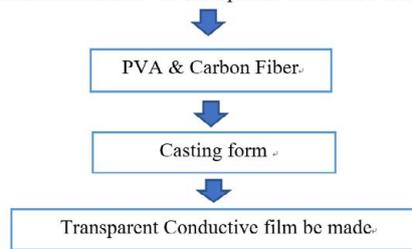
Figure 2: PVA transparent conductive film manufacturing process.
