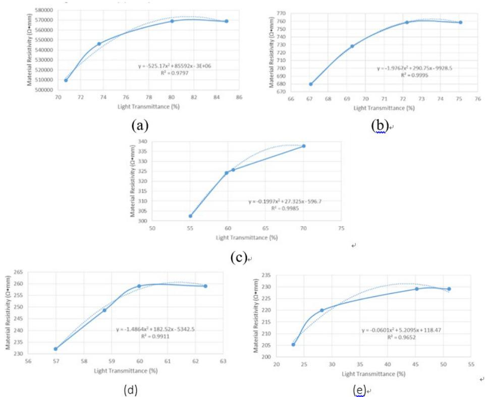
**Figure 10:** the relationship on the sample for Material Resistivity vs. Light Transmissivity with Equations. (a) Sample-01, CF:PVA of 0.1:30, (b) Sample-02, CF:PVA of 0.2:30, (c) Sample-03, CF:PVA of 0.3:30, (d) Sample-04, CF:PVA of 0.6:30, (e) Sample-05, CF:PVA of 1.0:30.
