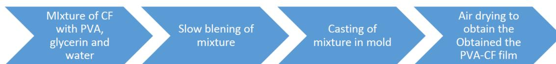
Figure 11: the process of fabricating PVA-CF transmittance conductive film.
