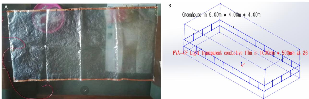
**Figure 15:** The PVA-CF Light Transparent conductive film be installed on greenhouse wall. (a) PVA-CF transparent conductive film. (b) Installation of 26 sheets of PVA-CF to the custom built agricultural greenhouse.
