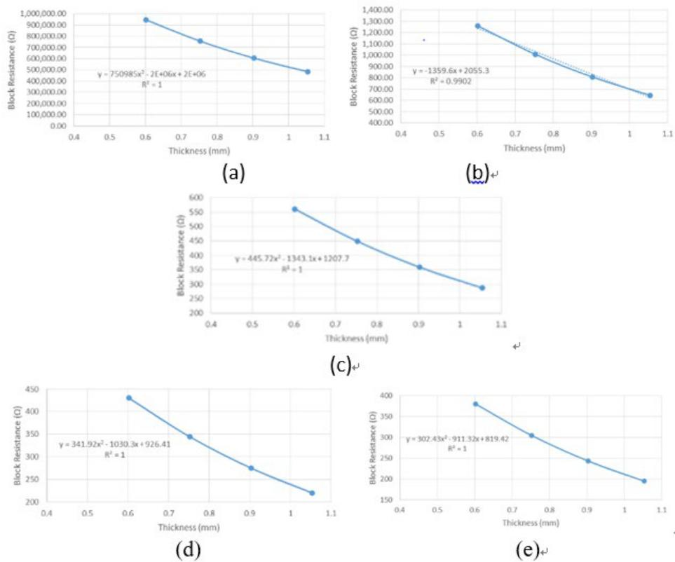
**Figure 7:** the relationship on the sample for Block Resistance (Ω) vs. Thickness (mm): (a) Sample-01: CF:PVA of 0.1:30 (0.33%), (b) Sample-02: CF:PVA of 0.2:30 (0.66%), (c) Sample-03: CF:PVA of 0.3:30 (1%), (d) Sample-04: CF:PVA of 0.6:30 (2%), and (e) Sample-05: CF:PVA of 1:30 (3.33%).
