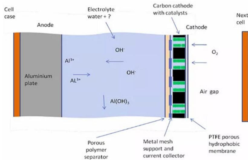
Figure 1: Schematic diagram of aluminum air battery.
