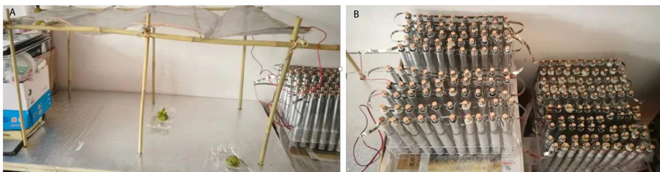
**Figure 14:** Aluminum-air batteries with  $K_2SO_4$  electrolyte (a) compose in 200 single aluminum air batteries with 12V and 20 mA for PVA-CF transparent conductive film, (b) To parallel connect 10 single battery and series connect 20 battery groups and all in one.
